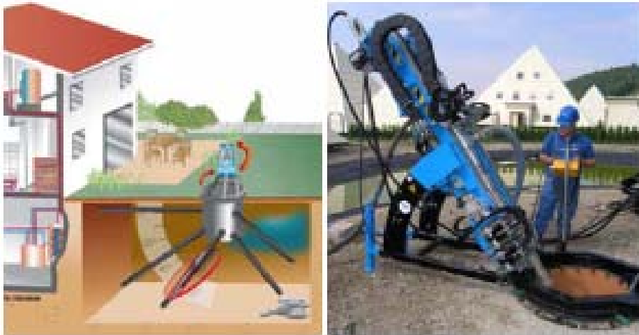
Figure 6. Geothermal radial drilling
