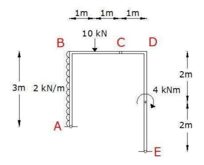
Figure 3. The frame structure used for trial one of the EAL-Tool.
