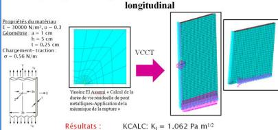
KCALC:  $K_I = 1.062 \text{ Pa m}^{1/2}$  $J-INT: K_1 = 1.0458 Pa m^{1/2}$ VCCT :  $K_I = 1.025 \text{ Pa m}^{1/2}$
